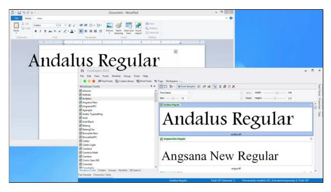
Customize text, width, height, and font size of the sample on the Face Sample bar and press Floating Sample ( ) button.
